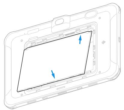
2. Slide the battery locks to secure the battery.
