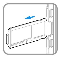
5. Place the nano-SIM card into the card holder tray with contacts facing down.
