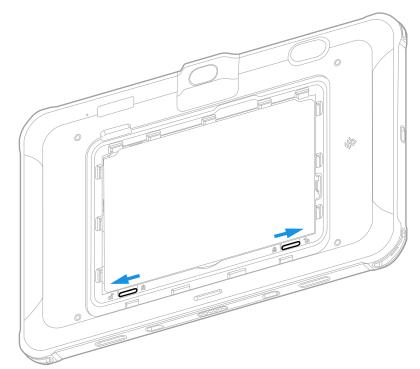
5. Pull up the tab on the back of the battery and use it to lift and remove the battery from the tablet.
