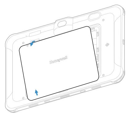
4. Slide the battery release latches to unlock the battery.
