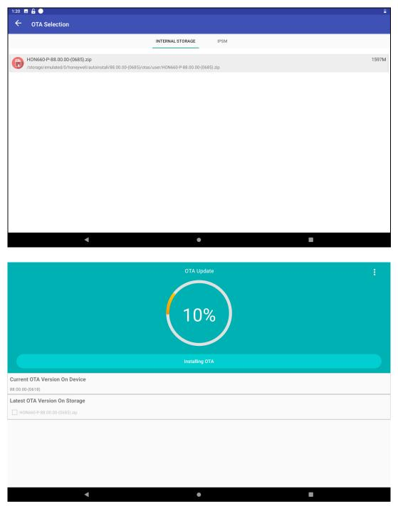
9. Once the installation is complete (100%), select **OK** when prompted to **Reboot** the computer. The computer reboots and finishes the update.
